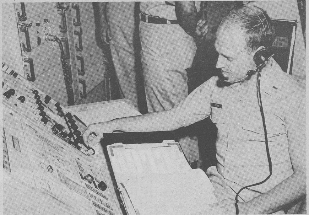
MANUAL CHECK -- Second Lt. Phillip S. Keenan uses his "Dash 1" check-list to verify his SAC high frequency radio communication settings.
